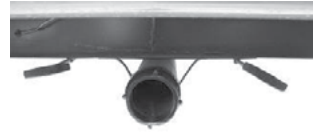
Black/Grey Tank Drain & Valves
