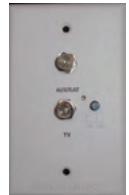
Antenna Power Supply
