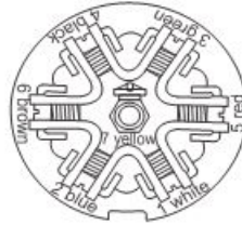
7-Way Trailer Plug- car end rear view
